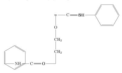
This illustrates the linkage between two MDI units via a polyether diol. In reality, the network is three-dimensional due to polyol functionality >2. The sodium bicarbonate does not alter the polymer backbone but contributes to cell formation via gas release. Fumed silica integrates into the matrix, providing nano-reinforcement at cell walls.
